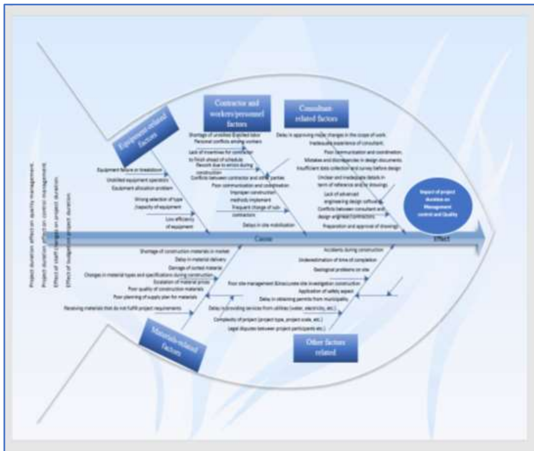
Figure 1.1: Fishbone Structure Shows Cause-Effect of Impact Project Duration
