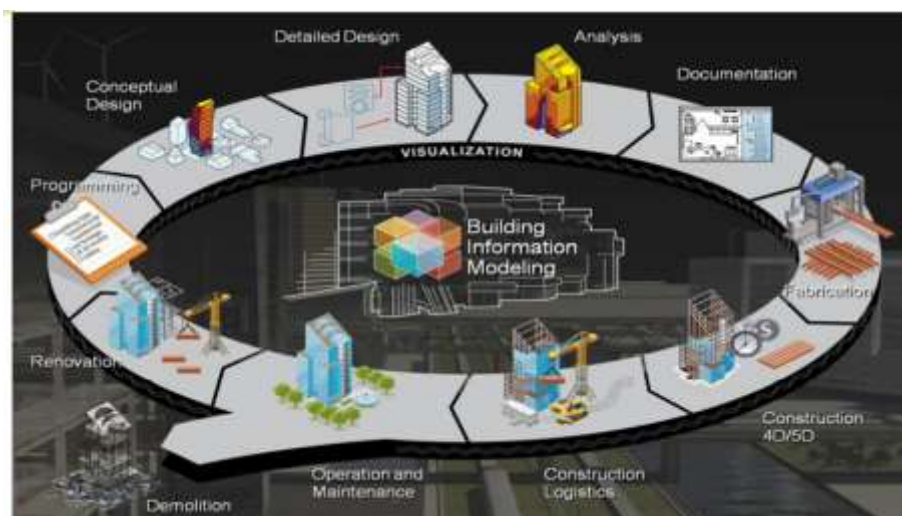
Figure 2.1: BIM used in the different construction lifecycle
