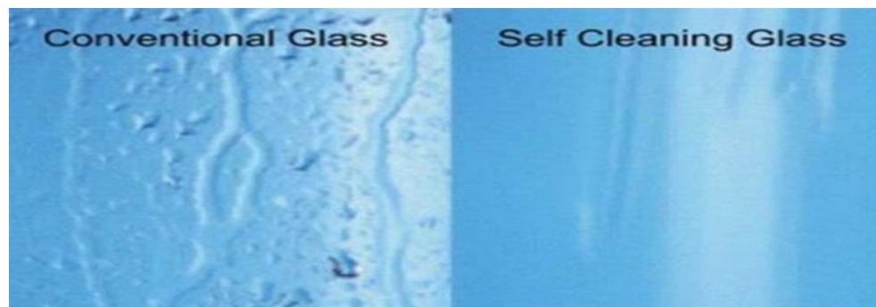
Figure 2.15: Comparison of Conventional and Self-Cleaning Glasses
