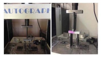
**Fig1 :** Destructive evaluation test, 3 Point bending test , to evaluate mechanial strength enhancement, [20]
