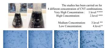
**Fig 2:** Effect of colloidal stability on CNT dispersions before application to samples of building material, searching the effect of Carbon nanotubes on mechanical strength of construction materials, [20]
