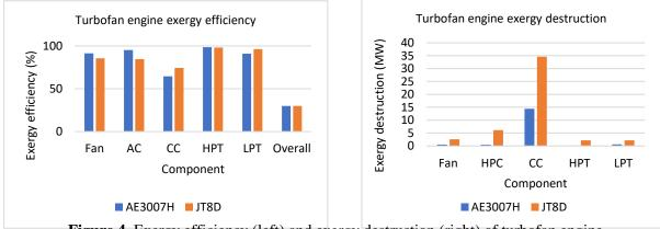
Figure 4. Exergy efficiency (left) and exergy destruction (right) of turbofan engine
