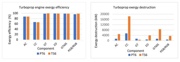
Figure 5. Exergy efficiency (left) and exergy destruction (right) of turboprop engine
