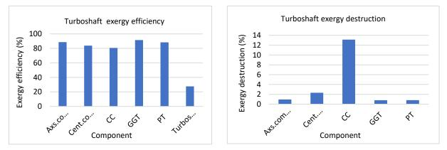
Figure 6. Exergy efficiency (left) and exergy destruction (right) of turboshaft engine
