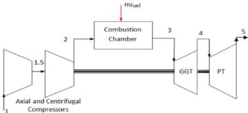
Figure 3. Schematic view of Makila1A1 turboshaft engine [7]
