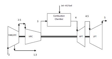
Figure 1. Schematic view of JT8D turbofan engine main components [7]
