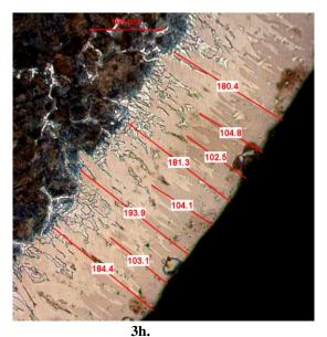
Figure 2. Boride layers formed on 34CrAlNi7 at 1223 K
