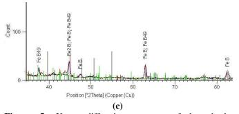
**Figure 5.** X-ray diffraction patterns of boronized 34CrAlNi7 (1h.) at different temperatures, a)1123K, b)1223K, c)1323K
