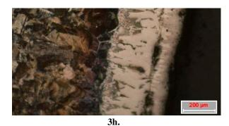
Figure 3. Boride layers formed on 34CrAlNi7 at 1323 K
