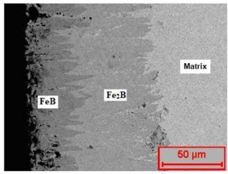
Figure 4. SEM (BE) image of boronized 34CrAlNi7
