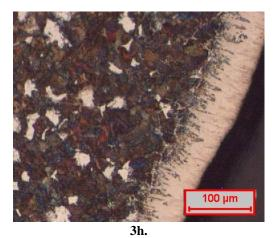
Figure 1. Boride layers formed on 34CrAlNi7 at 1123 K
