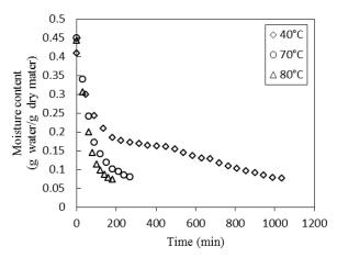
Figure 3. The spouted bed drying curve of rosehip.
