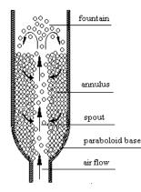
Figure 2. The spouted bed drying mechanism.
