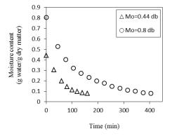
**Figure 5.** Effect of the initial moisture content on spouted bed drying of rosehip and variation of the drying rate for 0.44 and 0.8 initial moisture contents.
