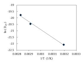
**Figure 7.** The influence of temperature on the effective diffusivity.
