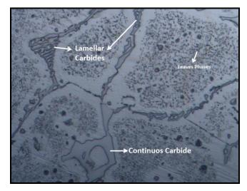
Figure 9. Microstructure of carbides near the macrocrack (200x - electrolytic etched with 6% chromic acid + 10% HCl)
