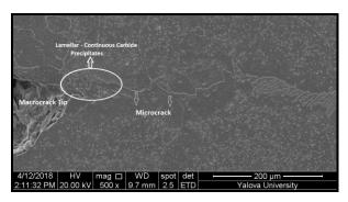
Figure 16. SEM image of macrocrack tip zone
