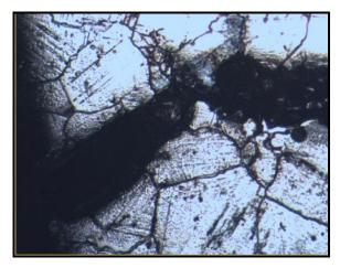
**Figure 11.** Microstructure of macrocrack origin (100x - e) electrolytic etched with 6% chromic acid + 10% HCl)
