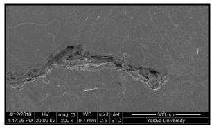
Figure 15. SEM image of macrocrack
