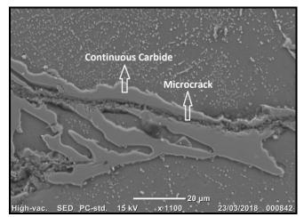
Figure 17. SEM image of microcrack
