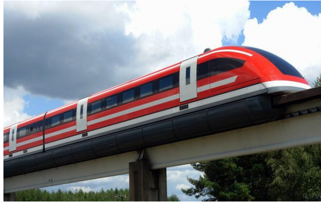
Figure 2.2: Transrapid 09 the Last Version of Transrapid Project With a Top Speed of 505 km/h.
